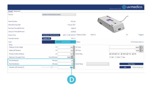
6) Add the "Maximum Occupant Time": how long the room is occupied during the duty cycle.
