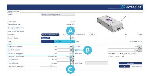
8) Change the intensity of the LED signal to the desired output.
